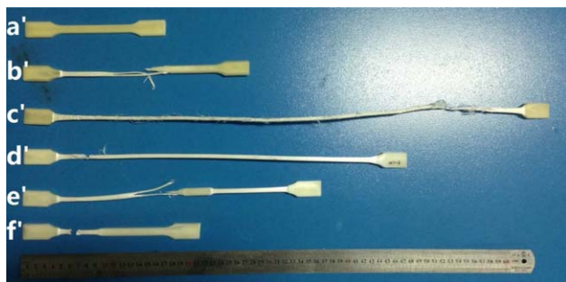
Figure 12. Optical images of the molded sample with different packing conditions before and after the tensile test. The first one (a') is the untested sample; the others (b'~f') are tested samples. The packing conditions were 10 MPa/1 s, 0 MPa/0 s, 10 MPa/1 s, 10 MPa/3 s, 30 MPa/1 s, and 30 MPa/3 s, respectively. [Color figure can be viewed in the online issue, which is available at wileyonlinelibrary.com .]
