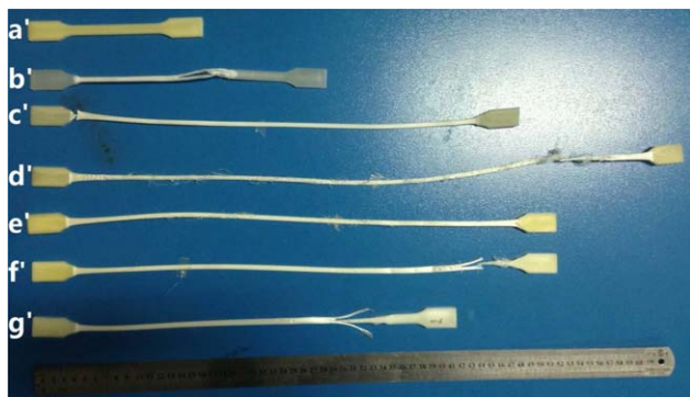
Figure 3. Pictures of the molded sample with different amounts of AC before and after the tensile test. The first one (a') is the untested sample; the others (b'~g') are tested samples. From top to bottom, the AC content by weight was 0.6%, 0%, 0.5%, 0.6%, 0.8%, 1.0%, and 2.0%. The length of the ruler is 60 cm. [Color figure can be viewed in the online issue, which is available at wileyonlinelibrary.com .]
